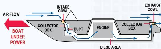
*All blower motors installed in exhaust ducts must be in working condition regardless of date of manufacture.*
